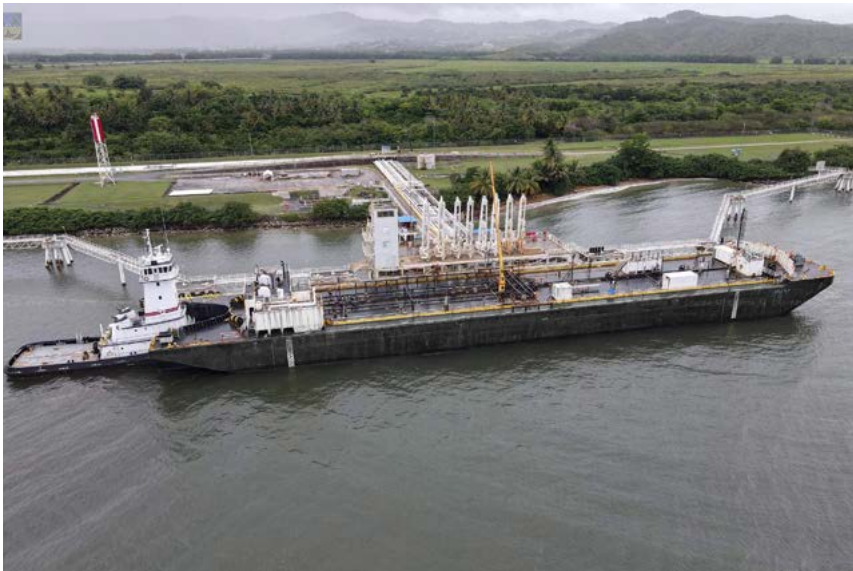
ATB unit, tug EMERY ZIDELL and barge DR. ROBERT J. BEALL, working in Yabucoa, Puerto Rico.
