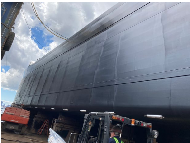
ATB barge ONEDREAM in drydock at Stabbert Marine Shipyard after receiving the final coat of antifoulant paint.
