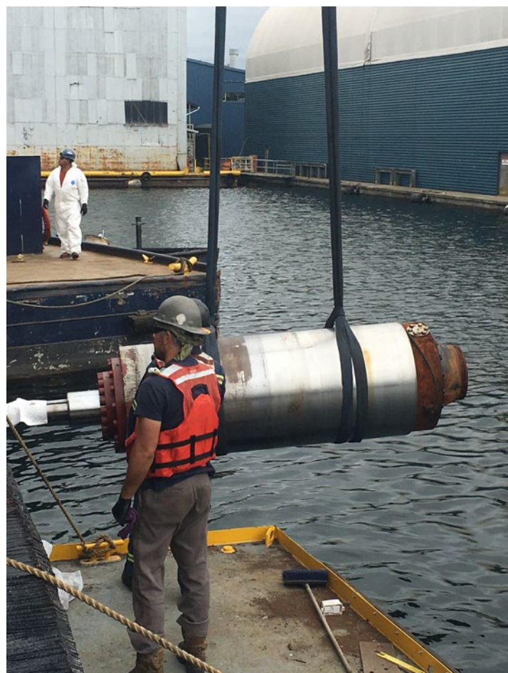
One of the Articouple pins being removed from the ATB tug MIN ZIDELL .
