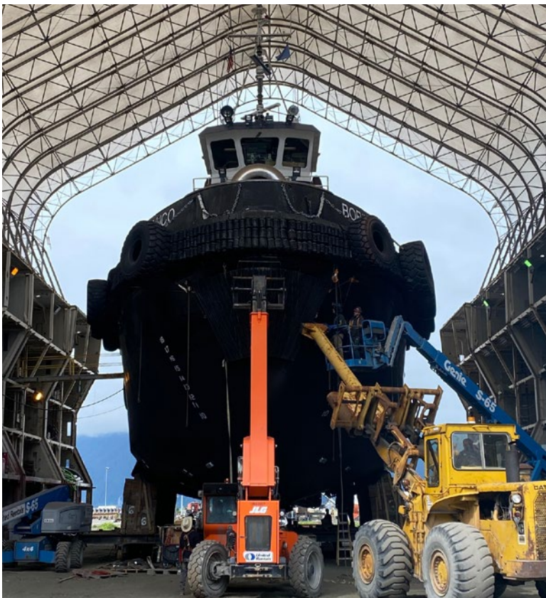
Tug BOB FRANCO at JAG Alaska Inc., Seward Shipyard in Seward, Alaska for a mid-term dry docking. The work completed included: painting, replacing anodes and transducers as well as some minor steel work near the keel coolers.
