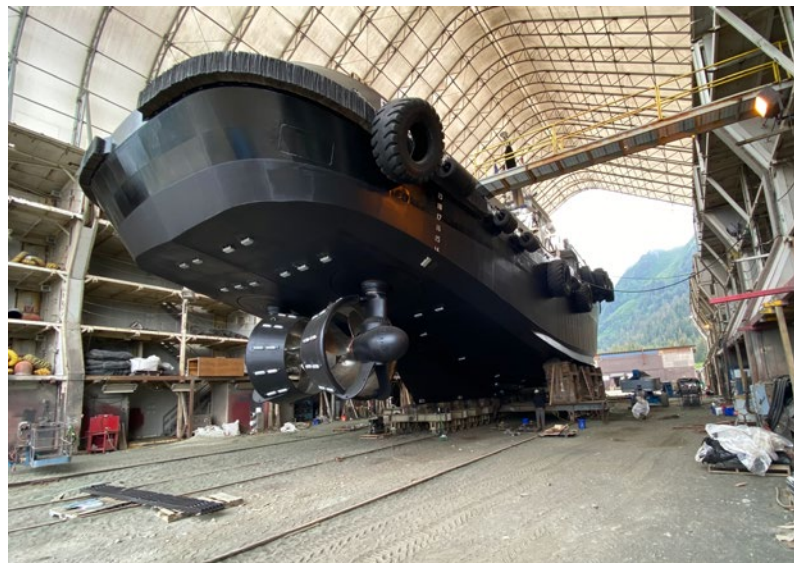
Tug BOB FRANCO at JAG Alaska Inc., Seward Shipyard in Seward, Alaska for a mid-term dry docking. The work completed included: painting, replacing anodes and transducers as well as some minor steel work near the keel coolers.
