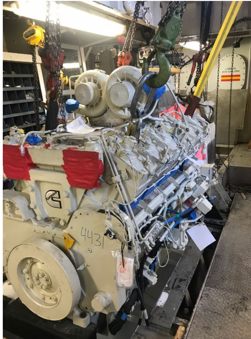
New Cummins QSK-38 Tier 3 engine inside the tug CE.
